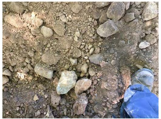
Photo No. 38 TP-05; excavated materials: fractured rock "blocks"
